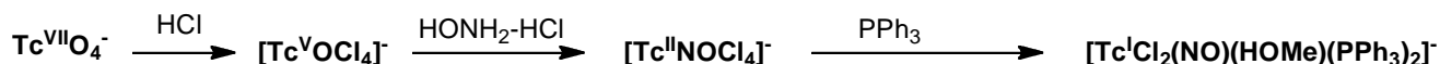
Figure 2: Sequential reduction reactions necessary to generate the Tc(I) -NO precursor [ Tc^I Cl_2(NO)(HOMe)(PPh_3)_2 ] from pertechnetate.
